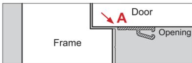
With the door open or closed, peel off the tape backing from the **Click** strip. Place the bottom of the Click strip on the horizontal baseline of the **door**. Line up the edge of the **Click** strip with the vertical mark on the **door** (A). When completely aligned on the vertical line, press the **Click** strip firmly into place.
